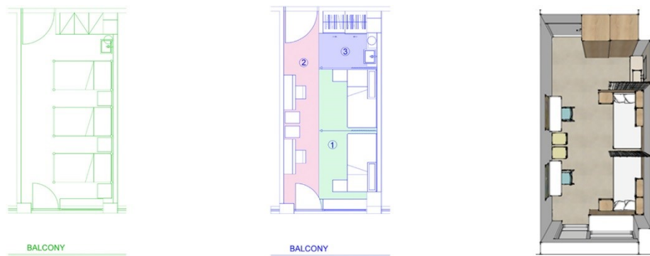
Figure 8 B - phase – changes under the STN and HBN. New floor plan under the STN (green color), new floor plan inspired by HBN and U.S. MHFDG: (blue color) with three (3) zones (1-rest/sleeping zone, 2-active zone, 3-private zone) and 3D floor plan (HBN and U.S. MHFDG) with used range of color and materials.
